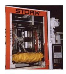
IPS Tie Bar Covers are used to protect your mouldings from unwanted tie bar grease contamination. A recent customer application using Tie Bar covers prevented labels getting into the tie bar bushings and causing excessive wear.
